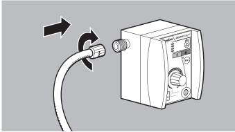
3. Connect the other end of the compressed gas tube to the device using the union nut. To do this, screw the union nut onto the device's compressed gas connection in a clockwise direction.
