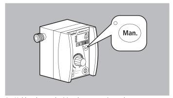
1. Hold and press the Man. button continuously.
