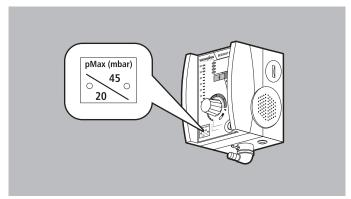
1. Press and hold the pMax button with control LEDs continuously.
