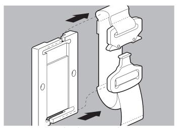
3. Remove the ends of the fastening strap from the depressions on the mounting plate.
