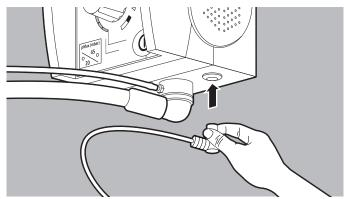
3. Connect the MEDUtrigger connector to the MEDUtrigger connection. To do this, insert the connector, without turning, straight into the socket.
