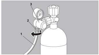
2. Using the union nut (2) or quick-release coupling, connect the compressed gas hose (1) to the pressure reducer (3) or central gas supply by hand. To this end, screw the union nut (2) clockwise.
