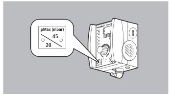
Set the ventilation pressure. To do this, press the pMax button with control LEDs.
