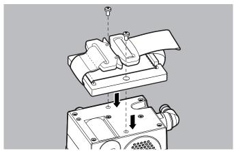
3. Screw the mounting plate onto the device by turning the supplied screws clockwise.
