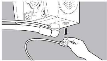
1. NOTICE! Material damage caused by twisting the MEDUtrigger connector back and forth!
