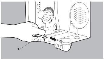
1. Grasp the end of the pressure measuring tube (1) and push onto the connection.
