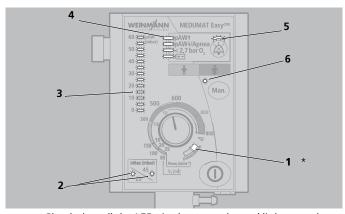
Check that all the LEDs in the control panel light up at least once when being switched on: Demand flow (1), pMax (2), ventilation pressure display (3), alarm (4), alarm mute (5), Man.(6).
