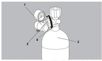
Connect the pressure reducer (1) to the oxygen cylinder (2). To
