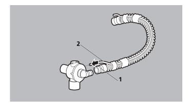
Connect the reusable ventilation hose (1) and pressure measuring tube (2) to the reusable patient valve.
