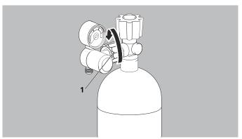
4. Remove the pressure reducer from the cylinder valve on the oxygen cylinder using the knurled union nut (1). To do so, turn the union nut counterclockwise.
