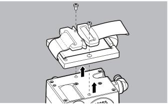
2. Remove the mounting plate. To do this, turn the screws counterclockwise out of the device.
