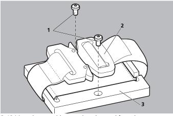
3-12 Mounting set with mounting plate and fastening strap
