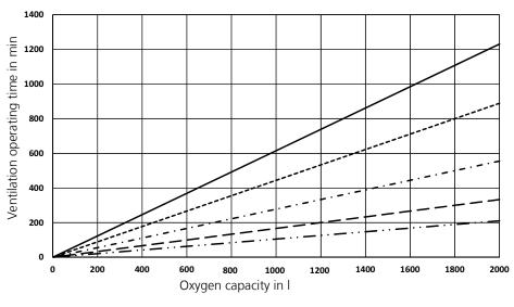
Freq. 25 bpm/V<sub>t</sub> 65 ml -----Freq. 15 bpm/V<sub>t</sub> 150 ml -  $\cdot$  - Freq. 12 bpm/V<sub>t</sub> 300 ml -  $\cdot$  - Freq. 10 bpm/V<sub>t</sub> 600 ml -  $\cdot$  · Freq. 10 bpm/V<sub>t</sub> 950 ml
