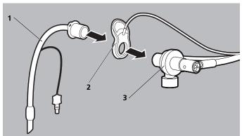
Connect the tube (1) together with the MEDUtrigger (2) on the patient valve (3).
