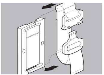
2. Insert the ends of the fastening strap into the depressions on the mounting plate.
