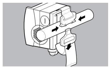
1. Hold the device securely and open the safety lock on the fastening strap. To do so, actuate both side levers at the same time and disconnect the buckles.
