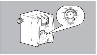
2. Turn the adjusting knob for ventilation parameters past the snap-in position in a counterclockwise direction.
