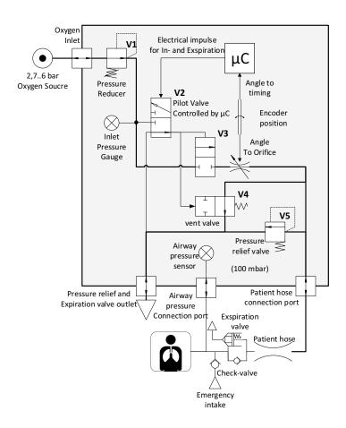
The pneumatic unit comprises the following components:
