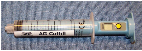
Figure 1 Photograph of the syringe device used in the current study. It provides a digital readout of the intracuff pressure.
